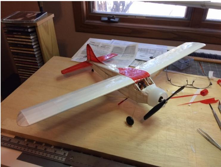
but after spending considerable time building it, and converting it from rubber band free flight to electric RC. I erred on the side of caution! It's a Guillows 24" Beaver that is now equipped with a Park 180 brushless motor, 10A ESC, 2 nano servos, a micro FASST receiver and a 2S 450mAHr Lipo. It weighs in at 4 oz.
